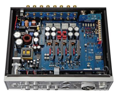
At centre lie four Class D amplifier modules, above them output network inductors and capacitors vital to Class D. At left is a large switch-mode power supply and at right the preamplifier board.
